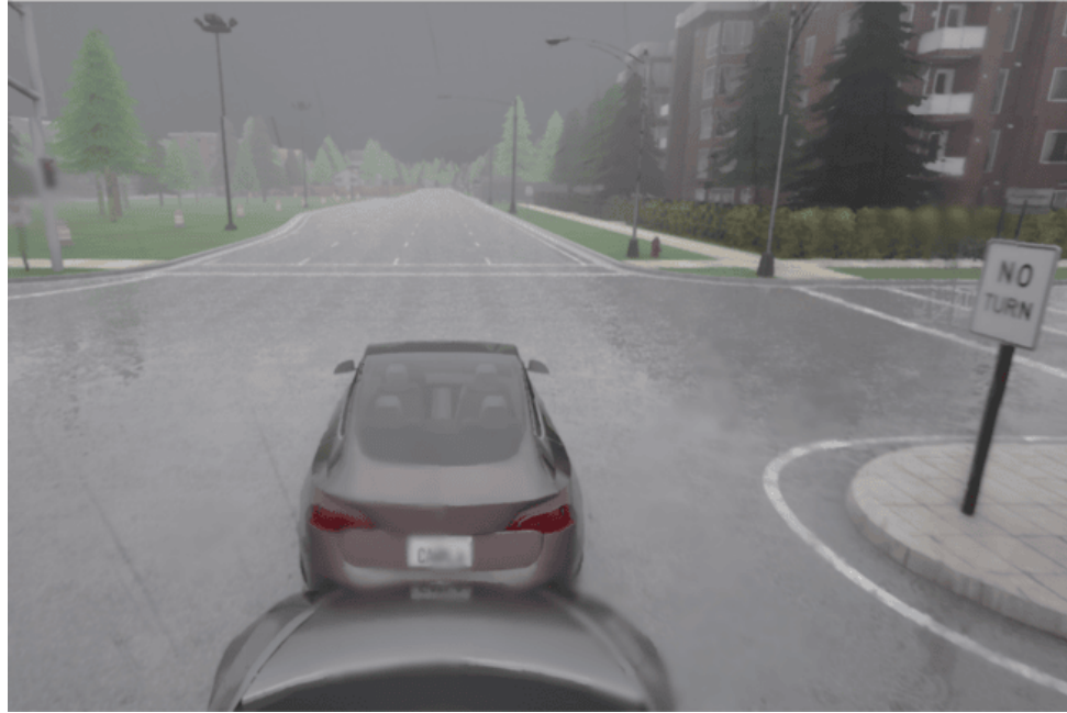
Figure 4. CARLA 0.9.15 In-Simulation View of the Dangerous Merge Scenario. A screenshot during execution shows the ego vehicle initiating a sharp merge into the lead vehicle's lane.
